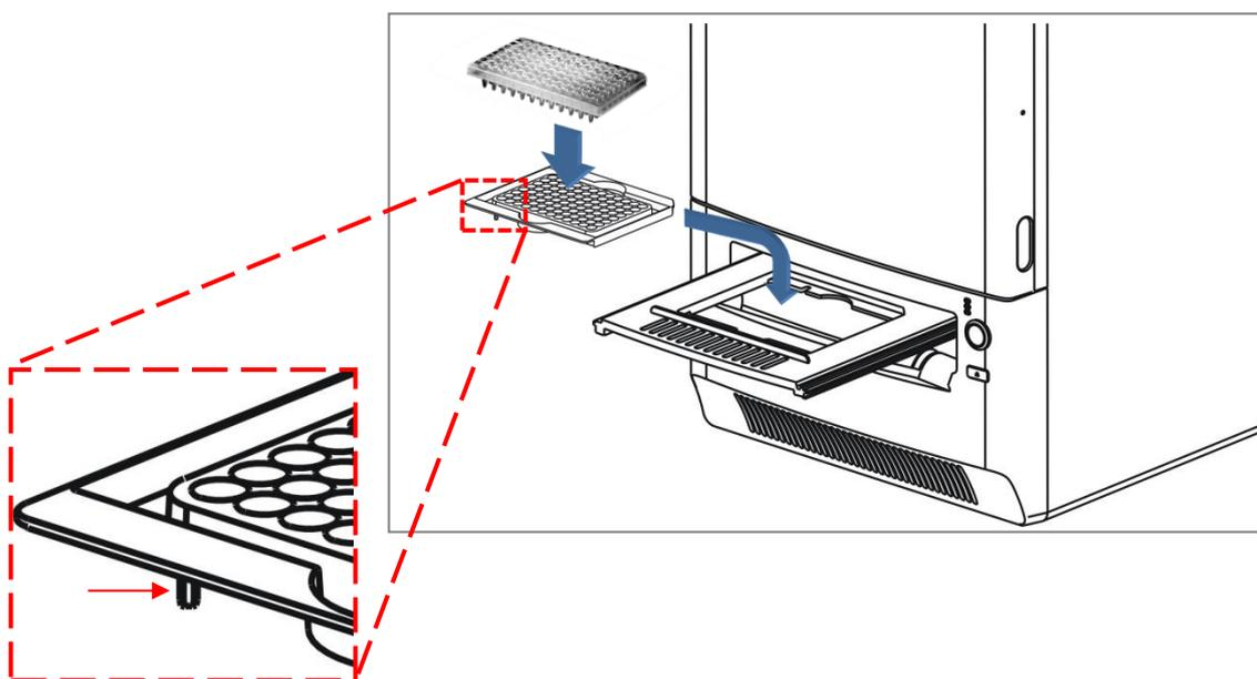
Figure 5. Alignment key on the plate carrier
