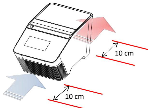
Please make sure there is no obstacle in the air flow path. At least 10 cm of space is required at the front and the back of the instrument.
